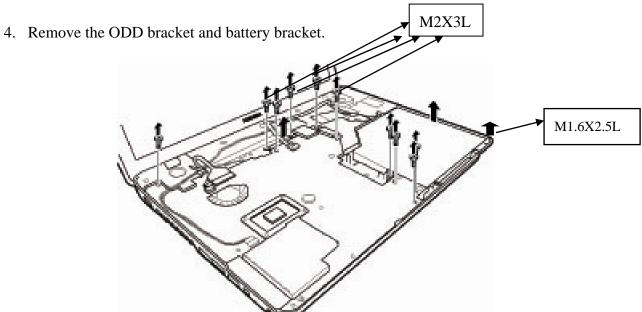
Figure 4-27 Removing screws secure the main PCB
